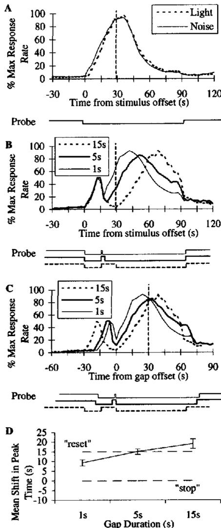
**Figure 5.** Timing in the gap procedure. Panel A: baseline probe trials. Panels B and C: reversed gap trials. Panel D: the rule used in reversed gap trials. Solid line = mean shift in peak time ( $\pm$  SEM) during reversed gap trials. Broken lines = predicted shift in peak time by stop and reset rules. The diagrams under the graphs depict the probe stimulus.
